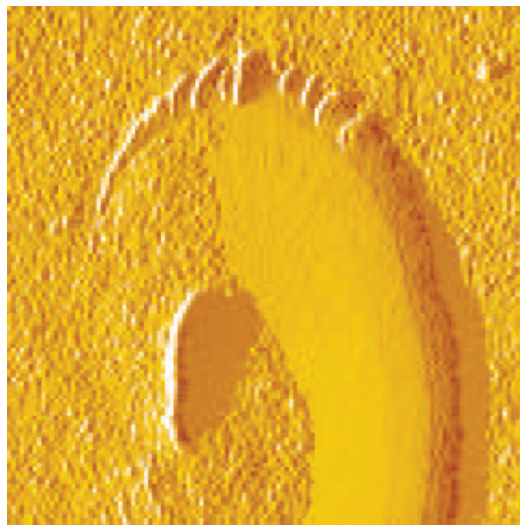
Figure 1. 1.6 \times 1.6 \mu\text{m}^2 AFM amplitude image of a polyethylene single crystal grown from the melt. The growth front was split at a certain distance into small branches twisted to form the spiral terraces in the same sense. The split pattern was formed on the course of quenching from isothermal condition at 120 °C to a coolant held at –90 °C. Sample was chemically etched to reveal the single crystal. 62
